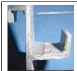
Evidence of obstruction – step in thrust surface
