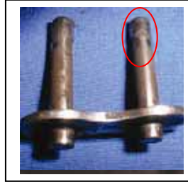
Evidence of overload – deformed pin deformed bushing
