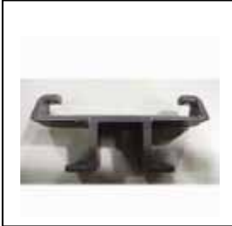
Evidence of uneven wear on top plate
